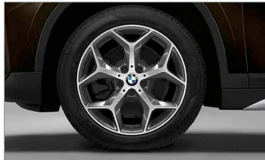
Y Spoke light alloy wheels (Style 569) 18 x 7.5 front and rear; and 225/50 front and rear run-flat all-season tires 1,2
